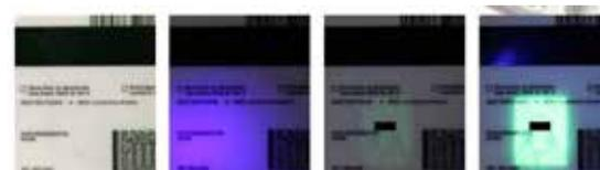
License security feature. In order: Normal light, competitor's "UV" light, competitor's "365nm UV light", and finally the Ni1UV 365nm light. (Ni1UV light source at 1 inches from subject). UV images at same exposure, no filter used.
